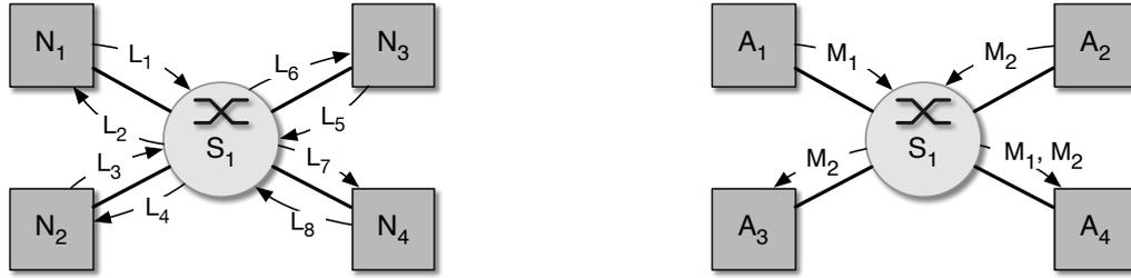
(a) Network with 4 nodes, 1 switch and 4 connections (8 links)
